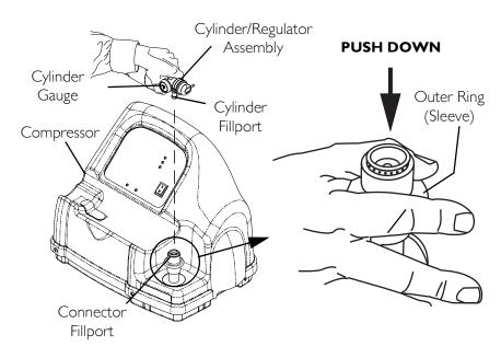
FIGURE 4.4 Disconnecting the Cylinder from the Compressor
